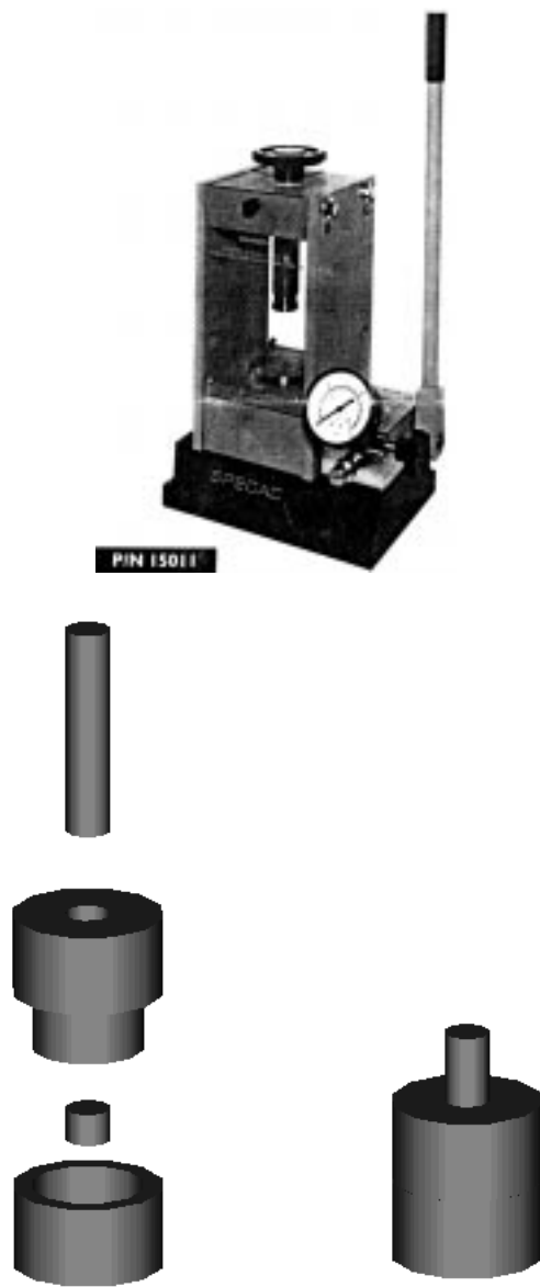
Fig. 1 Schematic diagram of the hydraulic press and dies used for compacting of powders
